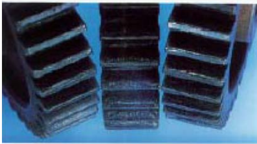
Heat Damage (burnt) Replace Gear set
